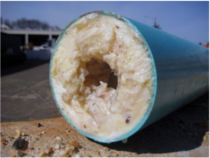
A sewer pipe clogged with kitchen fats, oils and greases.
