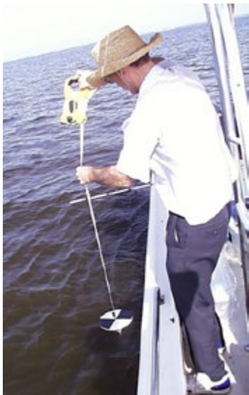
A scientist measures water clarity using a Secchi disk.
