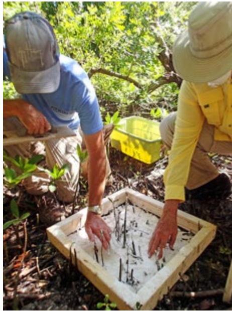
Biologists install a permanent feldspar marker to track elevation changes over time as part of the Critical Coastal Habitat Assessment. Photo by Lindsay Cross.
